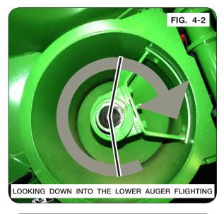
Using a safe lifting device rated at least 700 lbs., lift the auger and hanger bearing assembly up. Slowly lower the auger down through the auger plate opening to intersect with the drive bushing.
